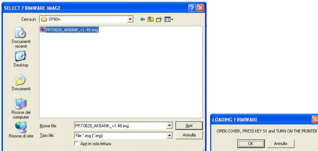
When select the **firmware.img** file and click on open key, an attention mask will appear to advise to power-on the printer in the special mode (open the cover and press ST1 key at power on).
