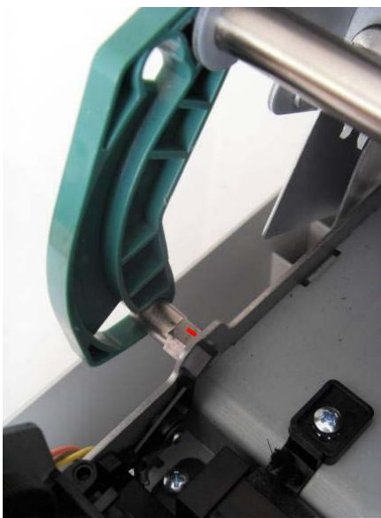
Fig. 8.1-8.2-8.3-8.4-8.5 - Print Head Gap adjustments
