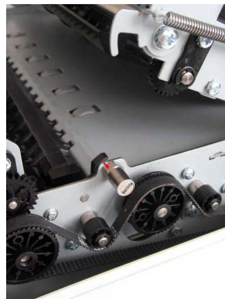
Fig. 8.1-8.2-8.3-8.4-8.5 - Print Head Gap adjustments
