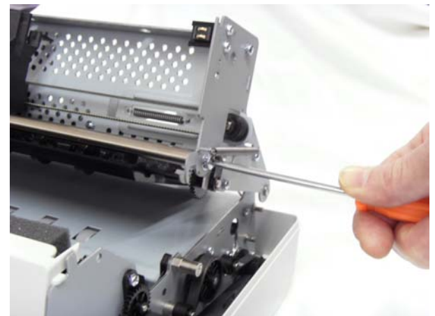
Figures 2.65-2.66-2.67-2.68 Carriage Assembly removal
