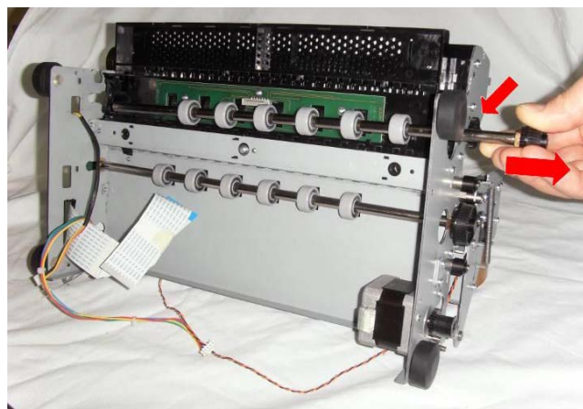
Figures 2.92-2.93-2.94 Front Lower Roller Assembly removal
