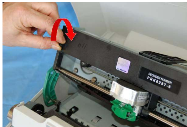
Figures 2.5-2.6-2.7-2.8-2.9 Ribbon Cartridge removal
