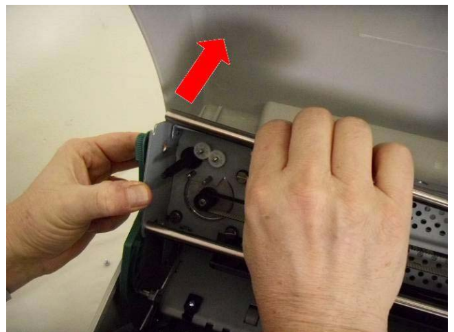
Figures 2.26-2.27-2.28-2.29 Ribbon Drive Gears removal
