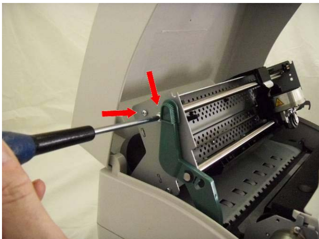
Figures 2.26-2.27-2.28-2.29 Ribbon Drive Gears removal
